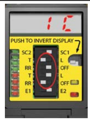
Figure 7-7. DIP switch programming to enable cascade installation
